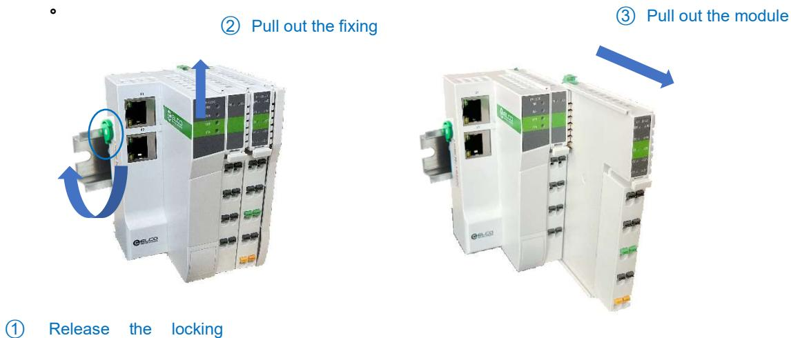
The wiring terminals of all modules can be removed separately to facilitate module replacement, as follows:
